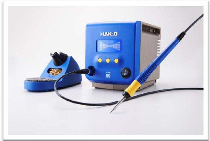
When you turn the soldering station on, it will perform a quick system check and display "Hello". Then the display will show you a graphic representation of the power output to the soldering iron tip as it heats to its predetermined temperature. The whole process is done in less than 10 seconds.
